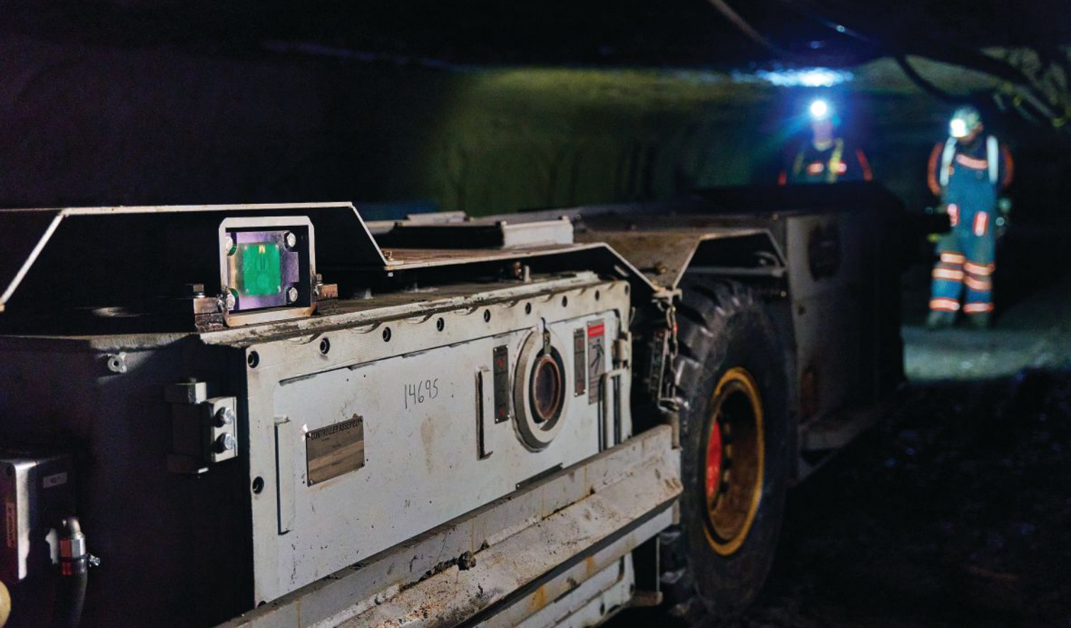
Guardian operates with a vehicular-mounted Command Unit and lightweight tags worn by miners.
